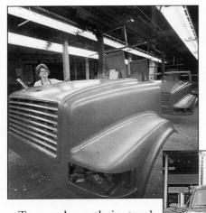
To produce their truck and personal watercraft components, a compression molding process is used. The key compound used in this process is Sheet Molding Compound (SMC) of which 32-34 million pounds
